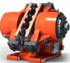
BSFI 300 Dualspring E-version Clamping force: 0 to 60.000 N Nominal braking force: 0 to 48.000 N*
